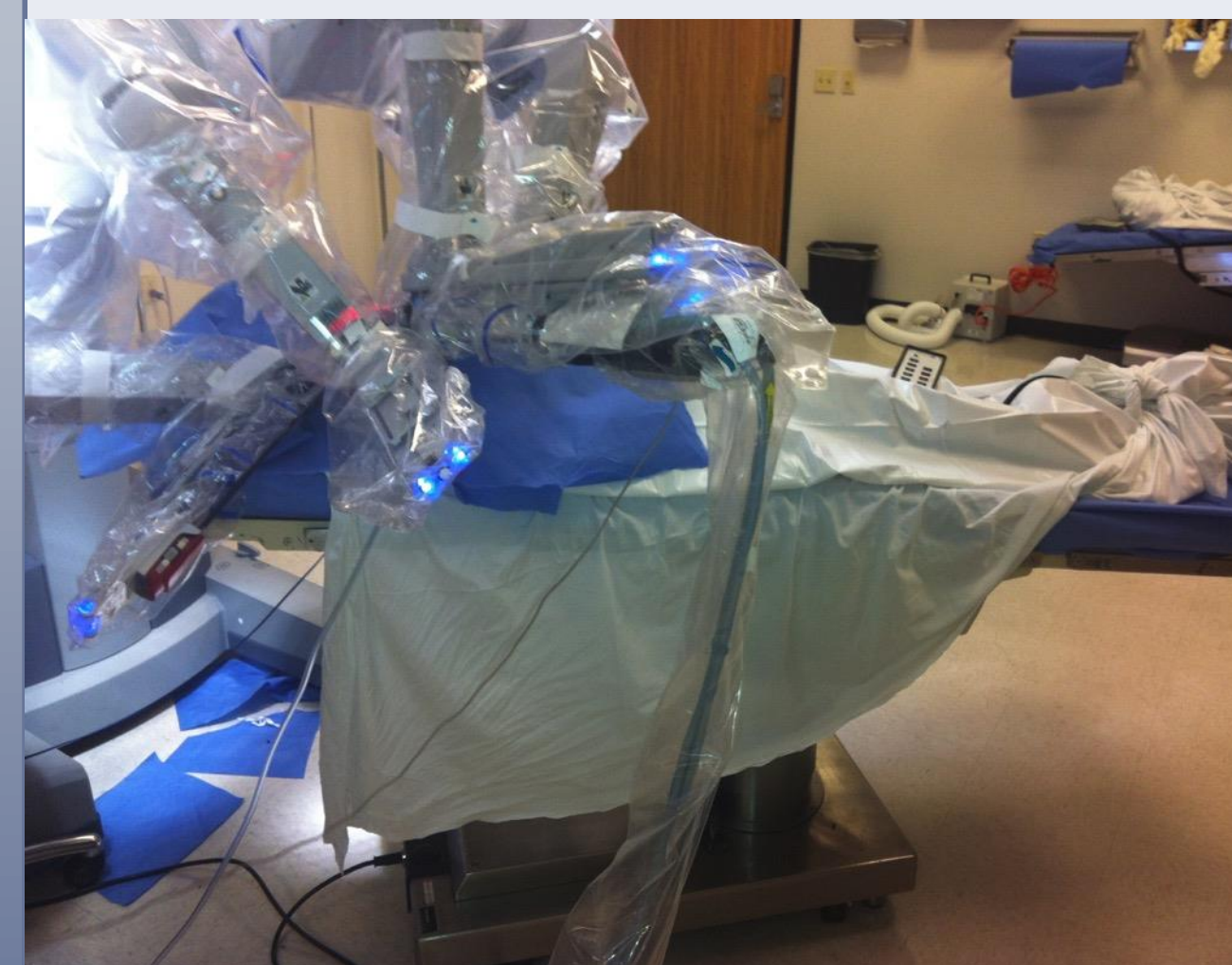
Figure 5. Surgical set up. Da Vinci robot arms in place and robot is positioned near the head of the bed. Four robotic arms were used in combination with three 8 mm instruments and camera.
