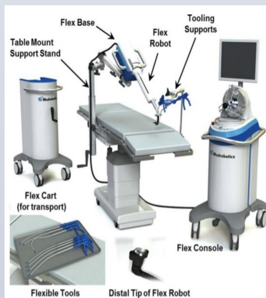
Figure 1. Operator controlled flexible endoscope with 50 individual linkages that can be advanced nonlinearly, using a joystick controller. Tooling support that for third-party 3.5 mm flexible instruments (Design Standards Corporation Charlestown, NH). The Flex Console houses controls and monitors. The reusable Flex Base converts electrical signals to mechanical movements. The disposable Flex Scope controls the motions of the endoscope 2 .
