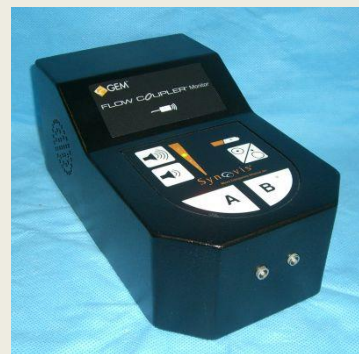
B) Ultrasonic microdoppler probe wire is inserted into monitoring box which is kept at patient's bedside. A and B channel allow for monitoring of two separate venous signals if necessary.
